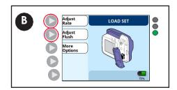
B. Press the **Adjust Rate** button or the **Adjust Flush** button and make any desired adjustments. (See Set Feed/Rate section below for additional information).
