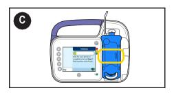
C. Once the air bubbles are out of the occlusion sensor region, restart feeding.
