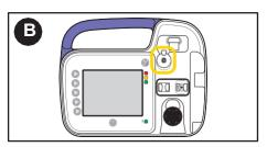
B. Check the valve actuator for blockages and confirm the valve actuator is correctly oriented.
