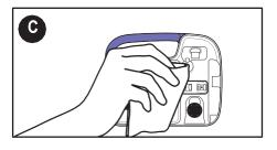
C. Clean and dry the Kangaroo OMNI™ Enteral Feeding Pump valve actuator.
