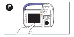
F. It alarm continues atter replacing Kangaroo OMNI™ Feeding Set, press **Power Off** to stop operation and use a different Kangaroo OMNI™ Enteral Feeding Pump.
