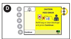
D. Upon priming, Kangaroo OMNI™ Enteral Feeding Pump will detect a Feed Error condition and alarm.
