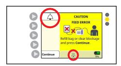
The alarms cannot be permanently silenced or muted. However, by pressing the Silence Alarm button, the alarm audio will be temporarily silenced for two minutes. After two minutes, the alarm audio will restart. To re-engage the audio alarm before the two minutes is up, press the Bell button. This will end the temporary audio pause, and restart the audible alarm.
