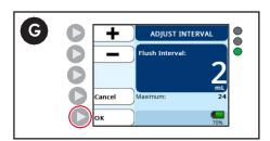
G. Press the **OK** button to confirm the time interval and return to the **Adjust Flush** screen.
