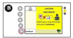
B. Press **Continue** and prime the pump to move the air bubbles or blockage through the tube. Disconnect patient from tubing before priming.
