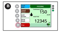
B. To change the rate or feed setting once feeding has started, press the **Stop** button.
