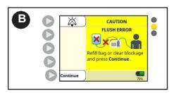
B. Press **Continue** and prime the pump to prepare for next flush. Disconnect patient from tubing before priming.
