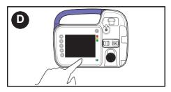
D. If alarm continues after replacing Kangaroo OMNI™ Feeding Set, press Power Off to stop operation and use a different Kangaroo OMNI™ Enteral Feeding Pump.
