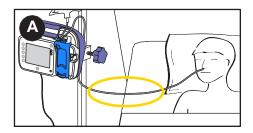
A. Check tubing between Kangaroo OMNI™ Enteral Feeding Pump and patient to locate the cause of the blockage and clear if possible.
