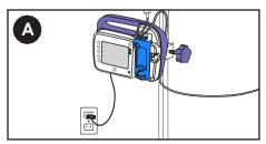
A. Plug Kangaroo OMNI™ Enteral Feeding Pump into a wall outlet for at least 12 hours to charge fully. Kangaroo OMNI™ Enteral Feeding Pump will automatically return to the screen that was active prior to the error and will continue to operate normally.
