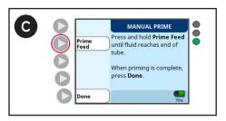
C. Press and hold the **Prime Feed** button until the feeding solution just begins to exit the distal connector.
