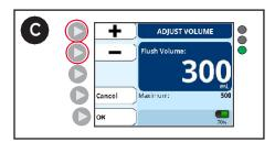
C. Press the + and – buttons to input the desired flush volume.
