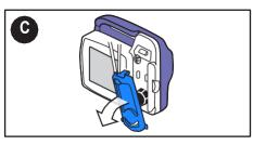
C. If alarm continues, **turn off pump** and **Remove** the cassette from Kangaroo OMNI™ Enteral Feeding Pump.
