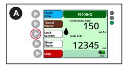
A. Press and hold the **Lock Screen** button for 5 seconds to lock the screen. **Note:** A countdown will appear to show how long to hold the button.
